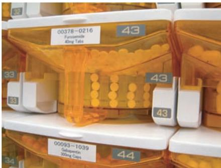
Factory calibrated cassettes do not require adjustments, and are more accurate than universal types.
