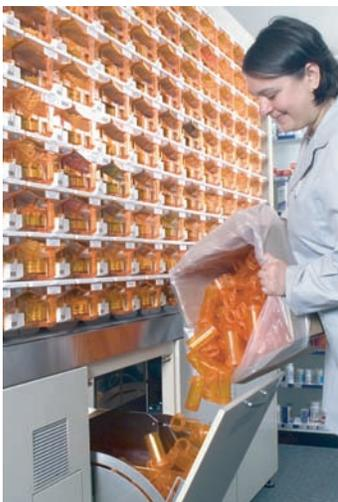
Vial bins are quick and easy to load by simply dumping in a box of vials.
