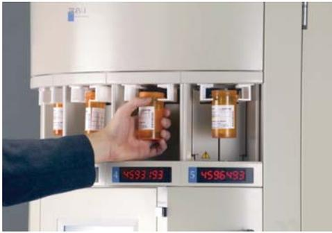
Pick-up windows display prescription number and barcode scanner confirms vial-picking accuracy.
